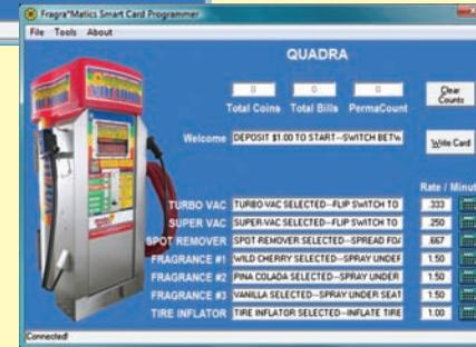
**2** Advance the text input cursor to each message field by pressing the "tab" key on your computer keyboard. Type the message you want to appear for each function on the machine.
